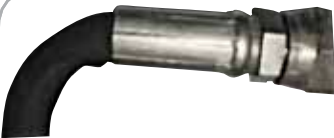
Hose bent too tight, damaged at end of coupling
