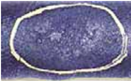
Hose with cover charred area from high heat or extreme aging due to heat or ozone
